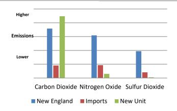
The production of electricity to support your product results in the emission of air pollutants such as carbon dioxide, nitrogen oxide, and sulfur dioxide. This graph compares the air emissions of (i) the regional system average, (ii) imports to New England, and (iii) a new natural gas power plant
