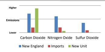
The production of electricity to support your product results in the emission of air pollutants such as carbon dioxide, nitrogen oxide, and sulfur dioxide. This graph compares the air emissions of (i) the regional system average, (ii) imports to New England, and (iii) a new natural gas power plant
